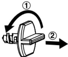
① Turn the packaging lock anticlockwise several times.
